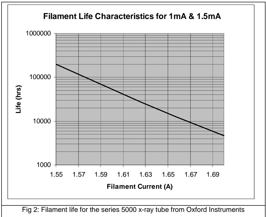
Fig 2: Filament life for the series 5000 x-ray tube from Oxford Instruments
