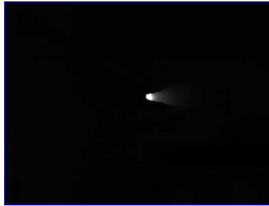
Figure 5: Conical smearing with increased exposure time of 10 ms.
