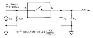
"Off" Isolation Test Circuit
