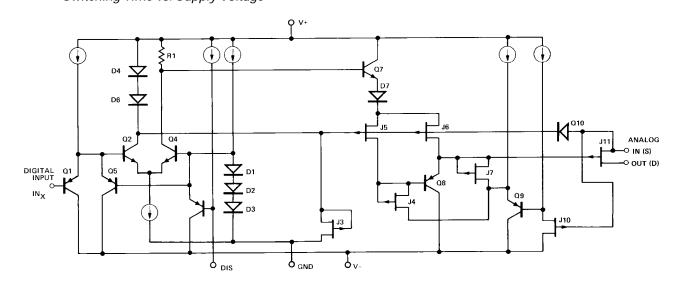
Simplified Schematic Diagram (Typical Switch)
