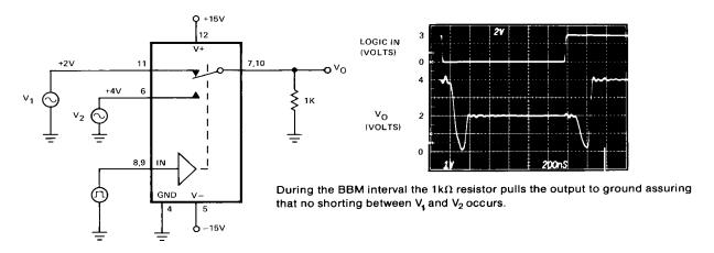
Single Pole Double Throw Selector Switch with Break-Before-Make Interval
