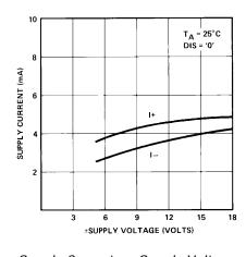
Supply Current vs. Supply Voltage
