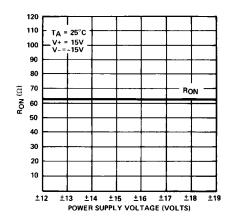
"ON" Resistance vs. Power Supply Voltage
