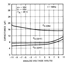
Switch Capacitance vs. Analog Voltage
