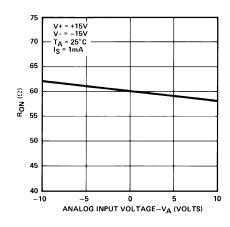
"ON" Resistance vs. Analog Voltage
