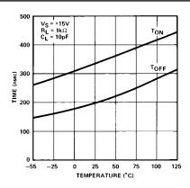
$T_{ON}/T_{OFF}$  Switching Response
