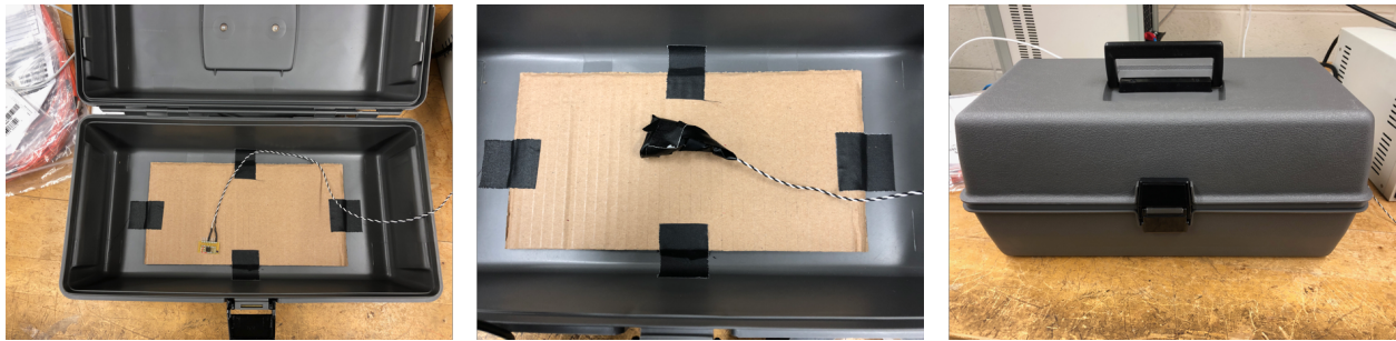
Figure 1 – From left to right: SiPM chip mounted on breadboard in toolbox, breadboard wrapped in fabric, closed box.
