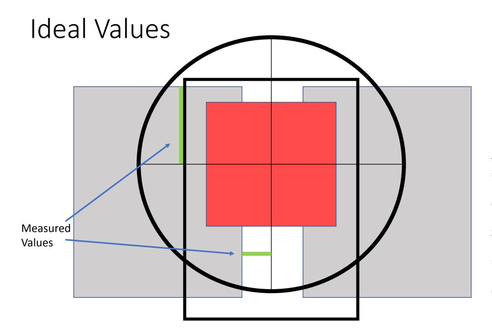
Pad height: 60mil = 1.524mm Package height: 170 mm Distance optical center to top of package: .63mm => Top of pads should be .542mm from center line of hole
