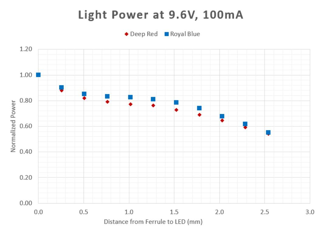
We found this to be true in our fiber tests. As shown above, percent of total power captured from each color stays high until around 2.2 mm, when the power captured begins to drop drastically. This is beneficial because it allows us to have some room for error and deformation in our setup.
