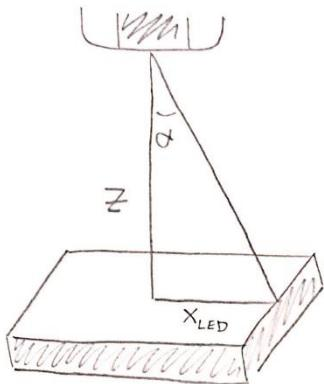
If the perpendicular distance between the fiber and the LED is less than or equal to  $z = x_{LED}/\tan(\alpha)$  where  $x_{LED}$  is the minimum distance between the center and the edge of the LED, the power captured will be constant. Up until this point, the LED fills the fiber's entire field of vision, so the  $1/r^2$  decrease in intensity cancels out with the increase in visible area.
